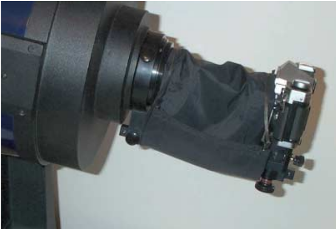
Figure 7. Next attach the Cloth Hood, if necessary. Using the wires on the Cloth Hood, wrap the wires around the Rail. Then [in most cases] the Cloth Hood can be draped over the eyepiece and camera.
