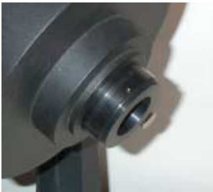
Figure 1. Attach the Rear Cell Adapter to Telescope
