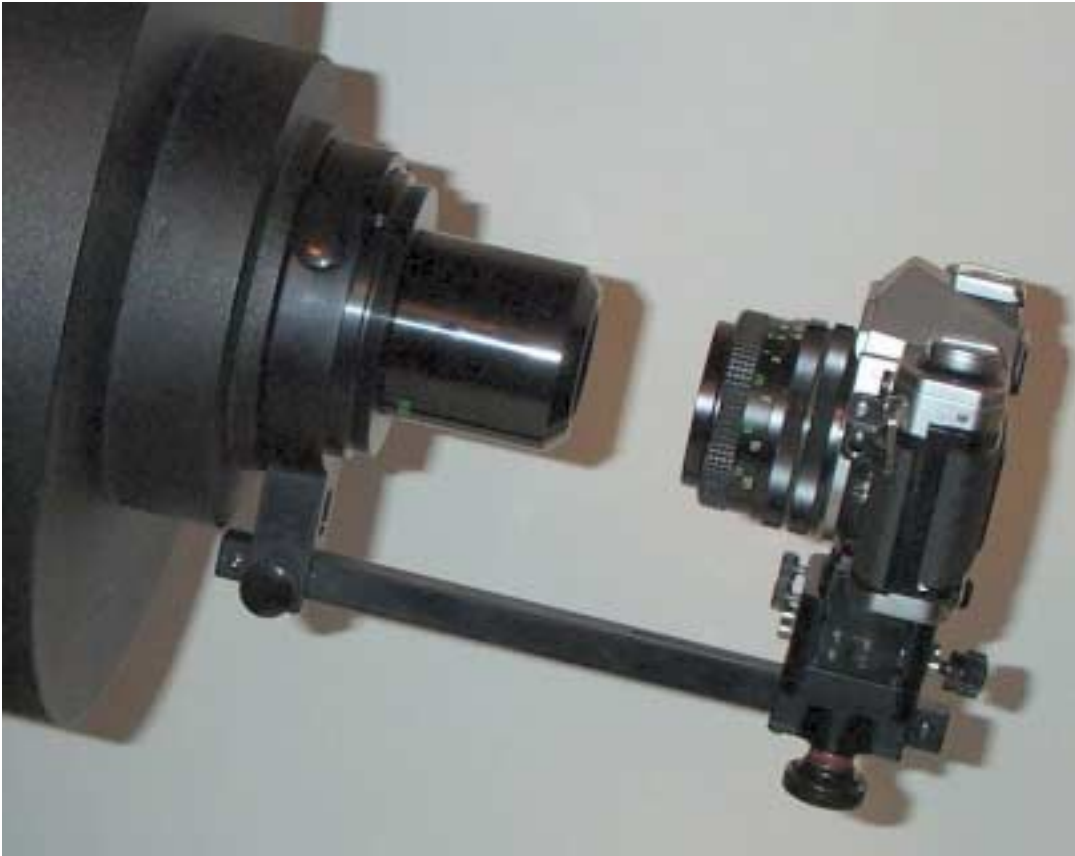
Figure 6. Attach the camera, or imaging device. Or another way of attaching the camera, is to mount it onto the Camera Platform, then slide the Camera Platform onto the Rail. At this point it will be necessary to center the camera. After the camera has been centered, tighten all the securing screws. Then move the Camera Platform up and down the Rail, while viewing, to get the desired Field Of View. Then lock the Camera Platform into position on the Rail.
